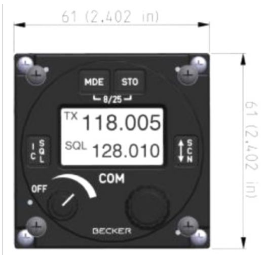
Figure 2-2: GT6201 front view, dimensions in mm and (inches)
